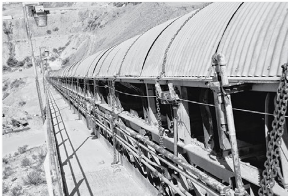
A conveyor belt system like this one takes copper ore to the smelter for the first round of processing.
