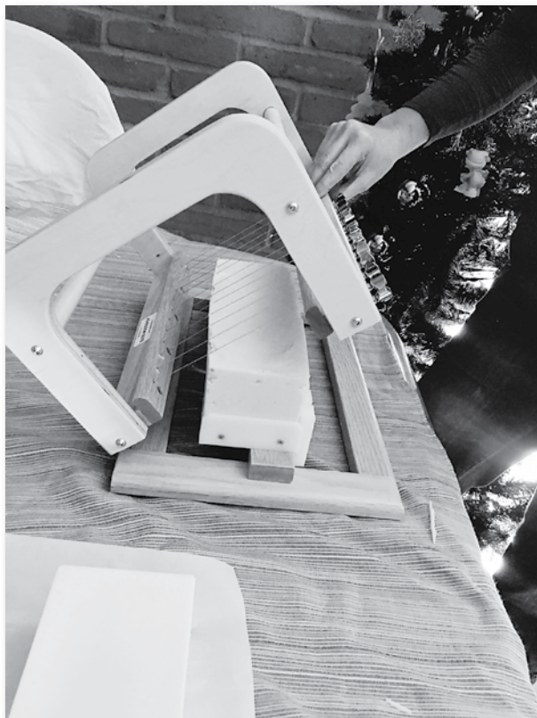
The block of soap is cut into bars.
