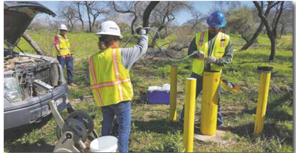
Purging the wells
